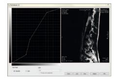
By using the gradation function you can individually optimize the image quality for each image source and printer.
